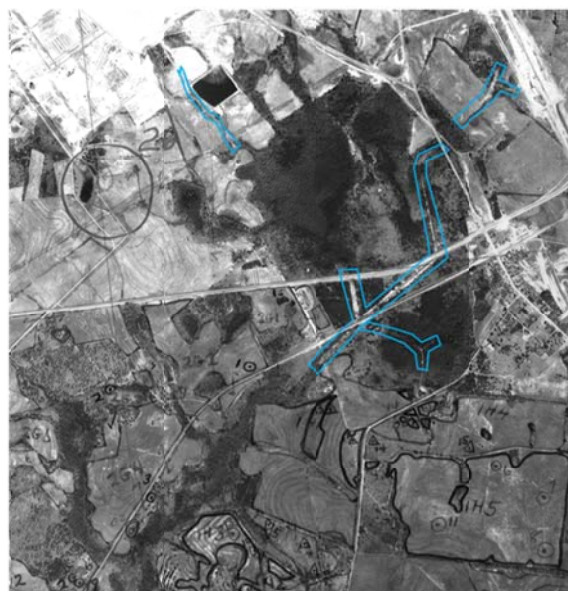
Figure 2. Meyers Branch 1956. Even though generally considered an undisturbed stream, the ephemeral headwaters was channelized between 1951 and 1956 to carry stormwater runoff from two industrial areas.
